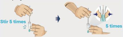
Remove the swab by rotating against the sample tube while squeezing the sides of the tube to release the liquid from the swab. Remove and discard the swab into waste bag provided.
